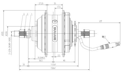
OLD: 113mm Shaft length: 158mm Motor cable length: L=250mm (optional)
